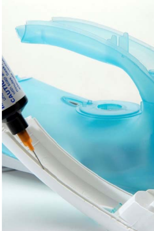
Figure 2 - Light curing adhesives bond many types of plastic
