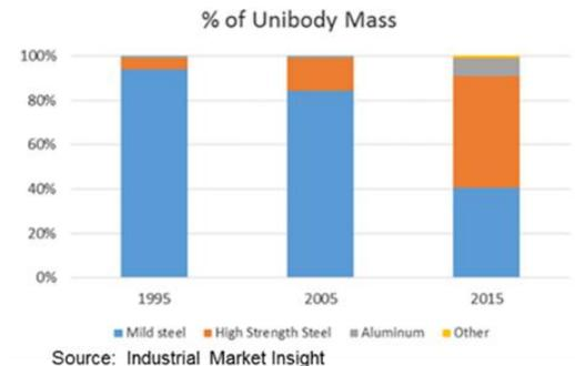
Structural adhesives have been a significant enabling technology in the industry's move to high strength steel. Because the density and elastic modulus of high strength steel is the same as mild steel, reduction in panel thickness, which is required to reduce weight, is accompanied by a decrease in stiffness. Structural adhesives have provided a solution
