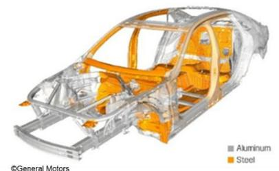
approach, enabled by adhesives and other advanced joining technology, was 250 pounds lighter than the base model, a savings of 7%.
