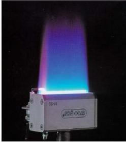
Flame treatment of the substrate surface for just a few seconds with an oxygen-containing (blue) propane or acetylene gas flame leads to the incorporation of oxygen-containing groups at the surface. This improves the wetting properties and hence the adhesion. Flame treatment is used almost exclusively for polyethylene and polypropylene substrates. The effect of the pretreatment subsides within a short time so that flame-treated substrates must be bonded immediately.
