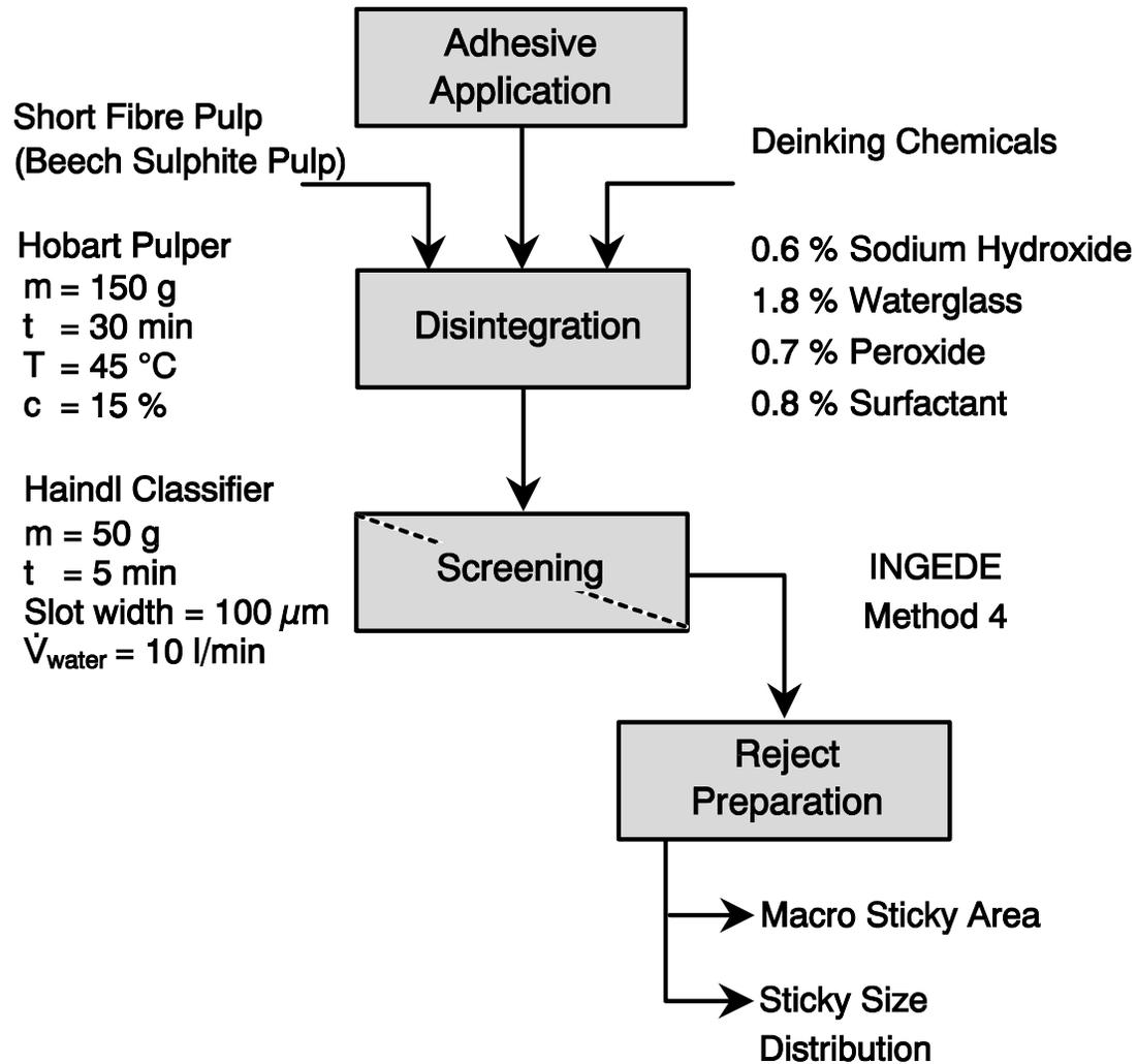
Fig. 5 Sticky Potential Test (INGEDE Method 12)
