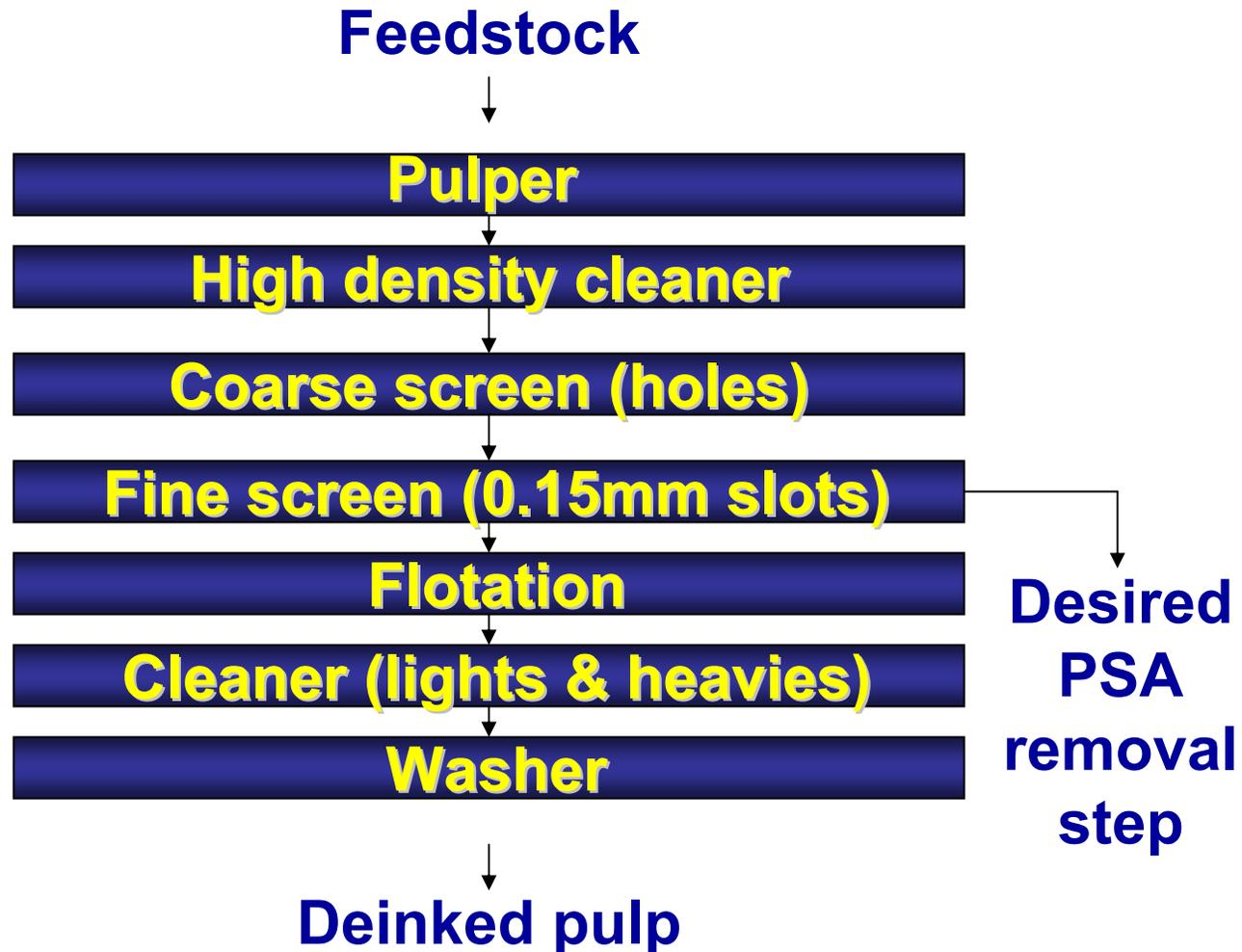
Fig. 3 External Paper Recycling Process
