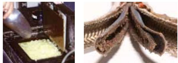
*Char caused by low/dry tanks and irregular filling impacts hoses, guns and end products*
