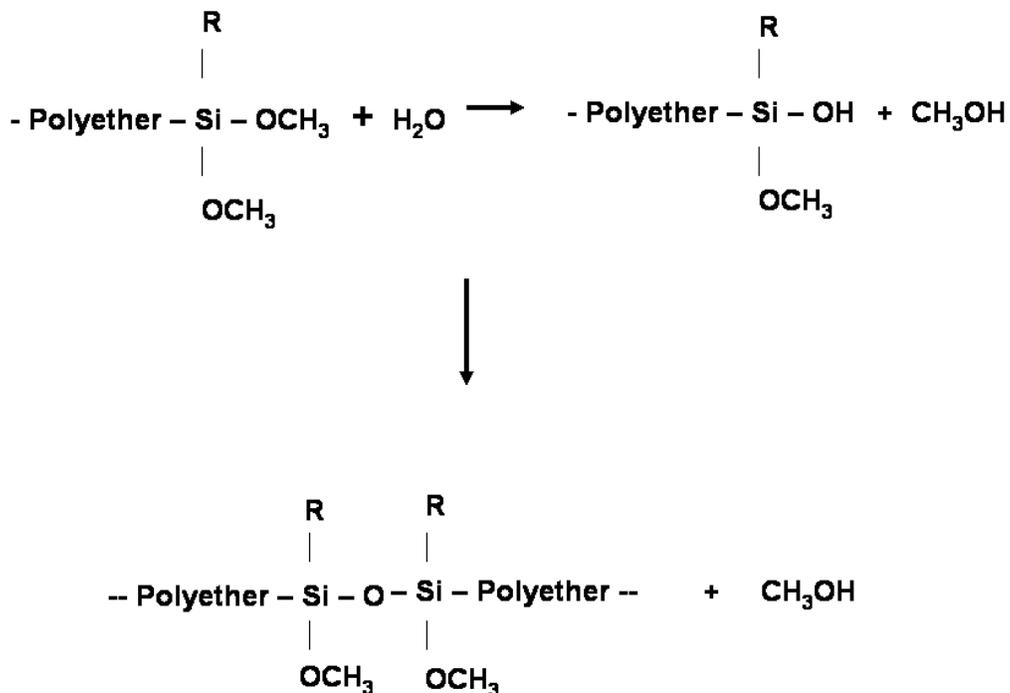
Similar to other sealants, MS polymers can be formulated with various plasticizers, fillers, and other additives to provide a wide range of properties depending on the application. Single-part formulations are most common, but two-part formulations are also possible.
