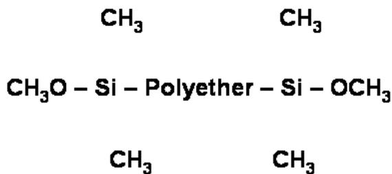
It does not have urethane, urea, or other functional groups that are typical in polyurethane sealants. MS polymer's polyether main chain provides low viscosity, low glass transition temperature, flexibility over a wide temperature range, and low color and odor. Since the main chain does not contain any highly cohesive segments, these polymers do not generally need solvent nor plasticizer.
