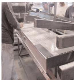
The customer was also having problems with the welding of shelf brackets for the truck bodies. When the sheet metal was welded, it created weld marks on the other side of the sheet metal. These cosmetic blemishes were being repaired before painting, adding to the total length of time it took to finish the truck body.
