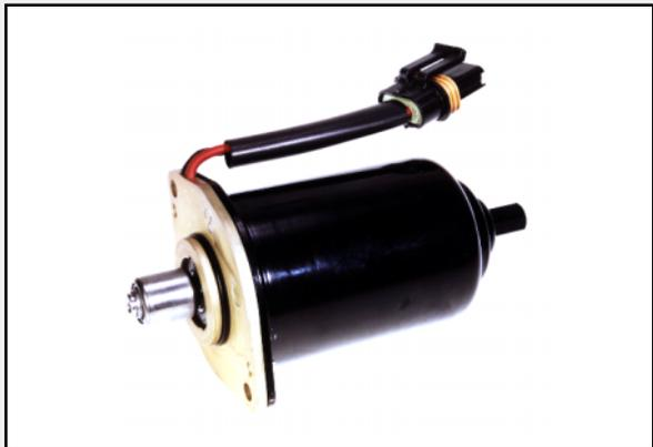
***Antilock Braking Motor. Loctite RTV sealant is used.***
