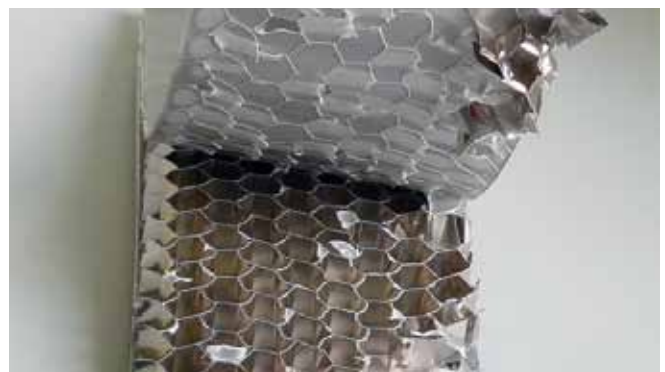
Figure 6: Peeled-off skin without pre-coating.
