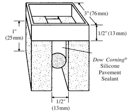
**Figure 2. Effect of Fuel Spill on Dow Corning® Silicone Joint Sealant**
